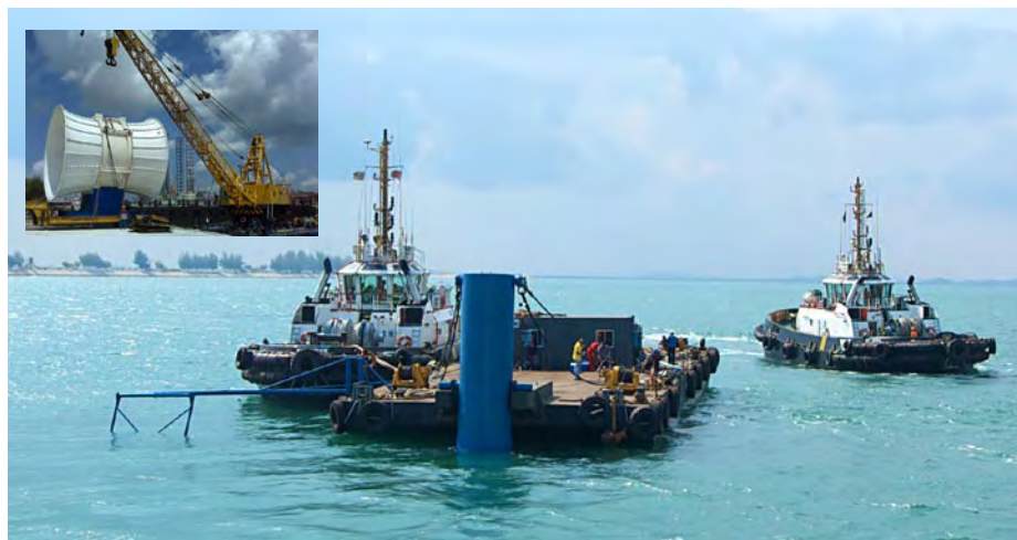
Drag race: the twin-tug towing rig and (inset) the Solon turbine being loaded for the tests off Singapore
